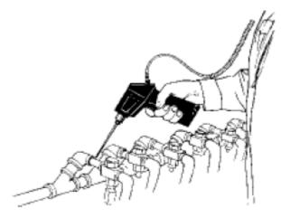
An ultrasonic test of steam traps is a positive test. The main advantage to ultrasonic testing is that it isolates the area being tested by eliminating confusing background noises. A user can quickly adjust to recognizing differences among various steam traps, of which there are three basic types: thermodynamic, mechanical and thermostatic (see Adca training Part 3).
