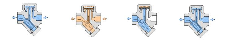
**INVERTED BUCKET ( IB )** traps usually fail in the open position because the trap loses its prime. This condition means a complete blow-through, not a partial loss. The trap will no longer operate intermittently. Aside from a continuous rushing sound, another clue for steam blow-through is the sound of the bucket clanging against the side of the trap.
