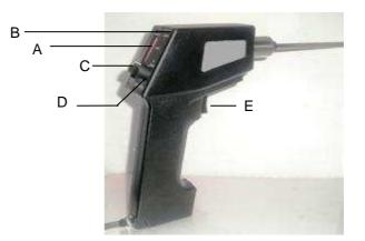
**A.** Bar graph Display: The display consists of a ten segment LED bar graph that will indicate ultrasonic signal strength. A low number of LEDs indicate a low level of ultrasound, conversely more intense ultrasonic signals will display more LEDs.
