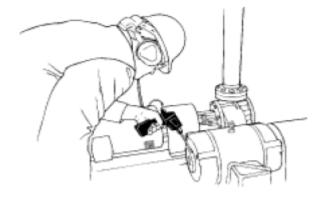
Ultrasonic inspection and monitoring of bearings is by far the most reliable method for detecting incipient bearing failure. The ultrasonic warning appears prior to a rise in temperature or an increase in low frequency vibration levels. Ultrasonic inspection of bearings is useful in recognizing:
